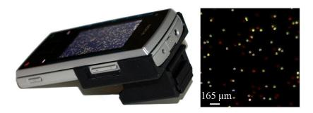
**Supplementary Figure 2.** (Left) Implementation of the same fluorescent microscopy principle on a different cell-phone model (Nokia X3, 3.2 MPixel) is presented. (Right) A mixture of green and red fluorescent beads that are imaged using the same unit shown on the left image.
