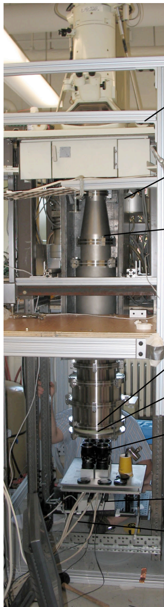
Supplementary Figure 2. Transmission electron microscope camera array (TEMCA). Key modifications enabling high-throughput EM image acquisition are labelled.
