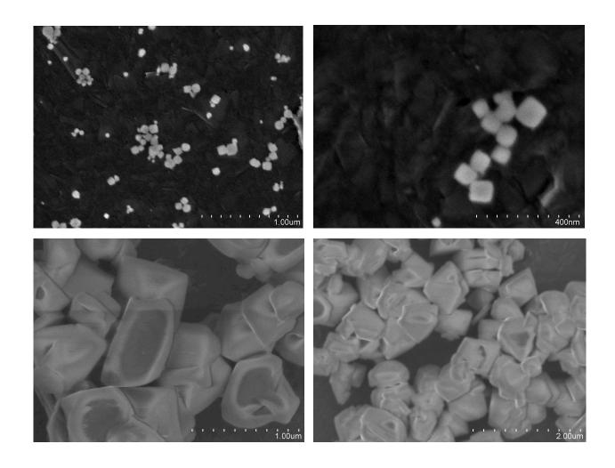
Figure S2. SEM images of nanocrystalline NaY (top) and NaY (Zeolyst) (bottom).
