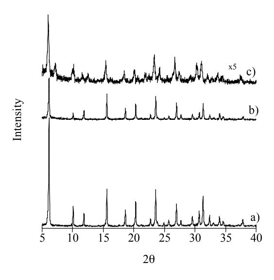
**Figure S1.** Powder X-ray diffraction pattern of a) NaY (Zeolyst) and b) NaY(Zeolyst) clicked with 4-Pentynol then Ga exchanged and c) nanocrystalline NaY. Impurity zeolite A is observed at  $2\theta$ =7.2° for the in-house synthesized NaY-nano.
