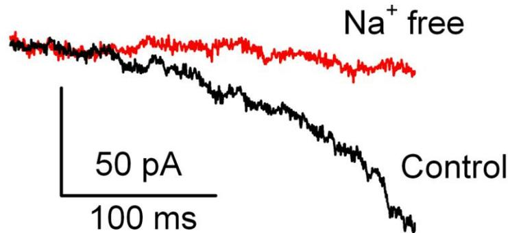
**Fig S4** The inward current elicited by ramp protocol was blocked when  $\text{Na}^+$  in the bath solution was replaced with  $\text{Li}^+$ , confirming that the inward currents largely were  $I_{\text{NCX}}$ .
