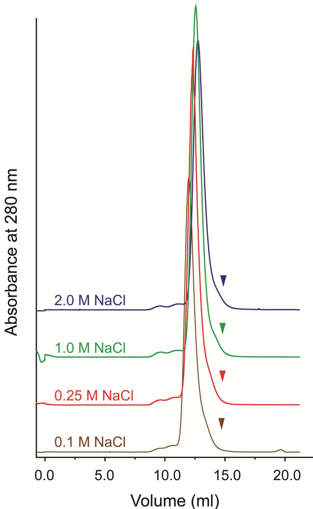
**Supplemental Figure S1** Stability of the NwCld dimer at different salt concentrations. The curves depict the absorbance (280 nm) trace of NwCld eluting from a Superdex 75 10/300 column at different salt concentrations. Arrowheads indicate the expected elution volume of an NwCld monomer. This elution volume was calculated based on the column calibration at the respective salt concentration.
