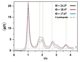
**Fig. S3.** Radial pair-correlation function  $\langle g(\bar{r}) \rangle$  for three  $\Theta$ s.
