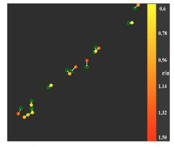
**Movie S2** String-like cooperative rearrangements of the most mobile particles at a GB ( $\Theta = 24.3^{\circ}$  and T = 299 K). The particle positions at t = 0 are shown by the hollow green circles and their final positions at  $t = t^{*}$  are shown by color-coded circles. The color code is according to the magnitude of their displacements. Movie S2 (MOV)
