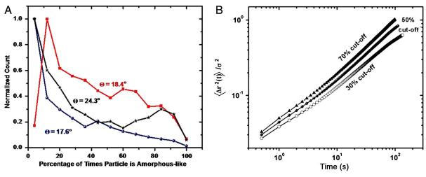
Fig. S1. (A) Frequency count of the fraction of time particles are amorphous-like for  $\Theta=24.3^\circ$  (black stars),  $\Theta=18.4^\circ$  (red squares),  $\Theta=17.6^\circ$  (blue circles). The dashed lines correspond to a fourth-order polynomial fit to the data. (B) MSDs rescaled by  $\sigma^2$ , for  $\Theta=24.3^\circ$  and T=299 K for three different temporal cut-offs.
