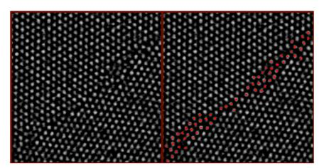
**Movie S1** Dynamics of colloids at a GB for  $\Theta = 24.3^{\circ}$  and T = 299 K. Raw data (*Left*) and the GB colloids (*Right*, marked in red) identified using the method mentioned in the main text.
