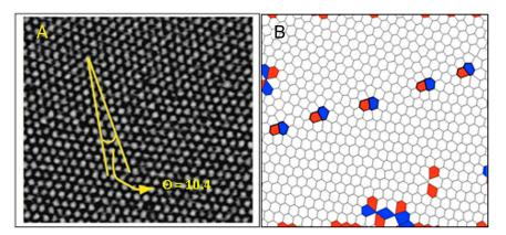
Fig. S2. (A) Image of LAGB. (B) Voronoi analysis of (A). The red and blue polygons along the GB correspond to the pentagon–heptagon pairs of the dislocation cores.
