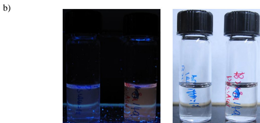
Figure S6. (a) UV-vis (dashed lines) and fluorescence (solid lines) spectra of taxoid-tetrazole 1 and taxoid-pyrazoline 1a . Compounds were dissolved in ACN/PBS (1:1) to derive concentrations of 25 \mu\text{M} . For fluorescence, \lambda_{\text{ex}} = 405 \text{ nm} . (b) Images of the two samples under 365-nm UV light (left) and ambient light (right). Left sample vial = taxoid-tetrazole 1 ; right sample vial = taxoid-pyrazoline 1a .
