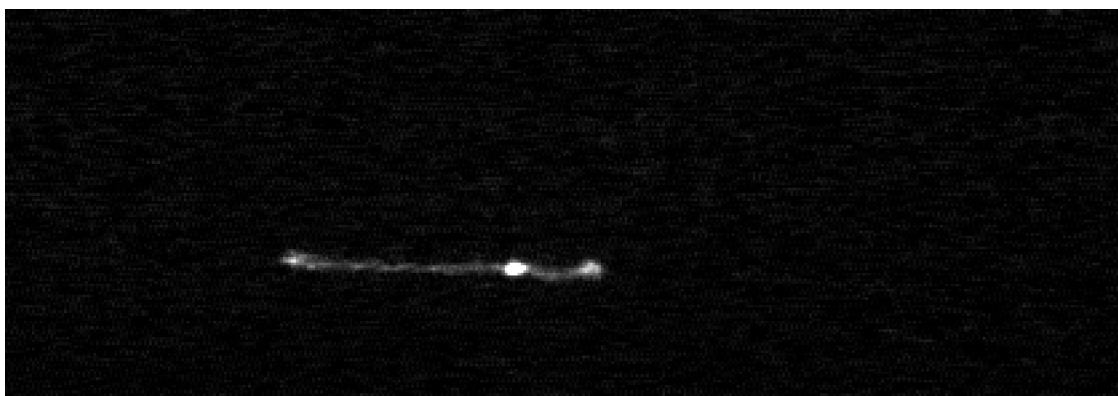
Movie S3. Electrophoretic stretching of a T4 DNA molecule that is initially compressed with an AC electric field of E_{rms} = 200 V/cm for 30 s in 0.5 \times TBE and in the cross-slot channel at a strain rate of 1.1 \text{ s}^{-1} .
