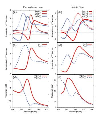
Supplementary Figure S1. Magnitudes and phases of dipoles extracted from Greens' function calculations of Au-Ag dimers for perpendicular and parallel polarization cases. (a-b) Real and imaginary parts of gold and silver polarizabilities, defined as  $\alpha$ =p/E<sub>ext</sub>, where p is the in-plane dipole moment and E<sub>ext</sub> is the external electric field. (c-d) Absolute values of polarizabilities. (e-f) Phases calculated as arguments of complex valued polarizabilities.
