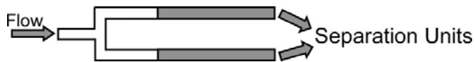
Fig. S3 Schematic of parallel separation device. Grey area is the multi perpendicular channel separation units, featuring 5 bottom inlets and channels. Main loading channel is 7.62 mm in length, 1 mm in width and 40 \mu m in height. Two branch channels are same in dimension (3.81 mm * 1 mm * 40 \mu m, l*w*h).
