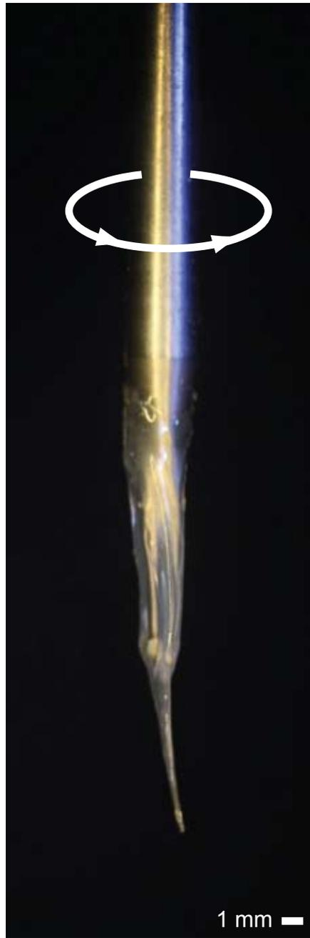
**Supplementary Figure 10.** The polishing whip tool. Tool is made by dipping drill bit into aquarium sealant, rapidly withdrawing it, and allowing it to cure. The whip is used to agitate the slurry of polishing grit and mACSF.
