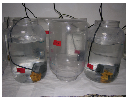
Fig. S4. Partial view of the experimental setup showing 3L experimental bottles containing individuals of Axinella spp. and a "Micra" water pump.
