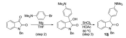
Step 2: The alcohol was prepared according to the general procedure using *N*-benzylisatin (237 mg, 1.00 mmol), 4-bromo-*N*,*N*-dimethylaniline (240 mg, 1.20 mmol), and Mg turnings (34.0 mg, 1.4 mmol). The reaction was conducted in THF (5 ml) for 1 h. The crude alcohol was taken on to the next step without
