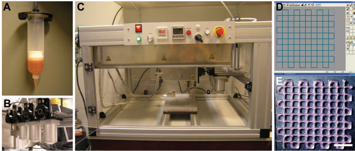
SUPPLEMENTARY FIG. S1. The components of the 3D fiber deposition technology. Hydrogel is loaded into the syringe (A), which is placed in one of the cartridges (B) on the BioScaffolder (C). Hydrogel fibers are deposited according to a model for a scaffold that is designed by the computer-aided design/computer-aided manufacturing software (D). Pressure-driven extrusion in a layered fashion yields porous 3D constructs (E). Scale bar: 500 \mu\text{m} . 3D, three-dimensional.
