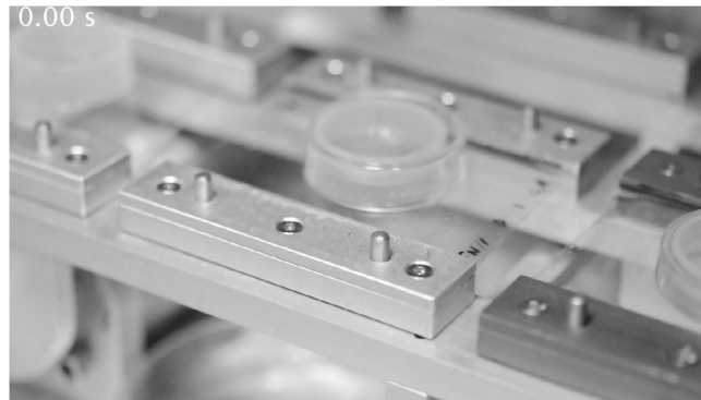
Movie S2. Representative video showing stretchers on our cyclic stretcher device subject to 20% strain. Movie S2 (AVI)
