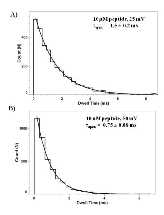
Single exponential fitting of open time histogram ( $k_{on}$  histogram) in the presence of the peptide at A) 25 mV and B) 50 mV. Experimental conditions are 1M KCl, 20 mM MES, pH 6.
