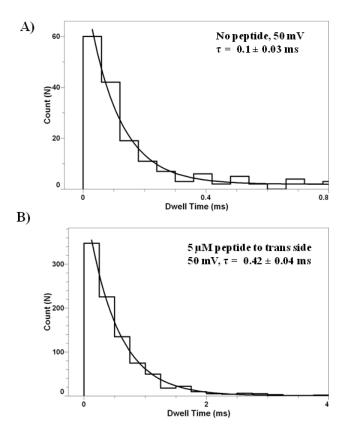
Single exponential fitting of blockage time histogram in the A) absence and B) presence of the peptide. Experimental conditions are 150 mM KCl, 10 mM MES, pH 6.
