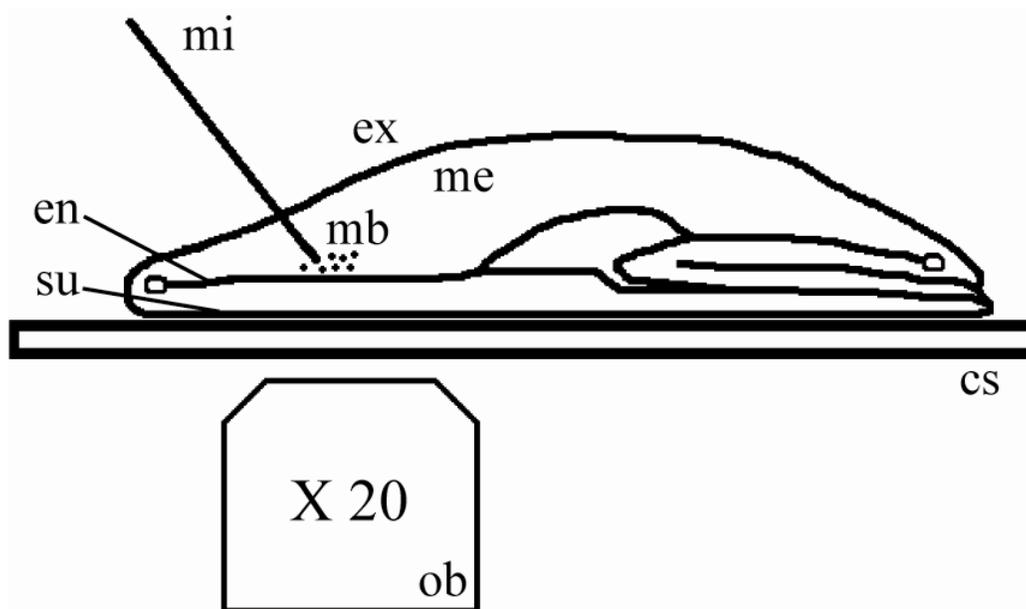
FIGURE S1 Schematic views of the set up used for *in vivo* microbeads injection in the mesoglea of an anesthetized juvenile jellyfish for microrheology experiments. For clarity, the diagram does not show actual sizes of the elements. Cover slip (*cs*); endoderm (*en*); exumbrella (*ex*); microbeads (*mb*); mesoglea (*me*); micropipette (*mi*); objective (*ob*); subumbrella (*su*).
