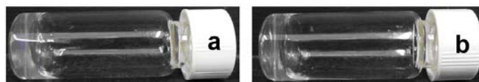
Figure S3. Optical images of (a) 1T +deoxyadenosine ( \text{A}_{10} ) mixed gel; (b) 3T +deoxyadenosine ( \text{A}_{10} ) mixed gel triggered by alkaline phosphatase.
