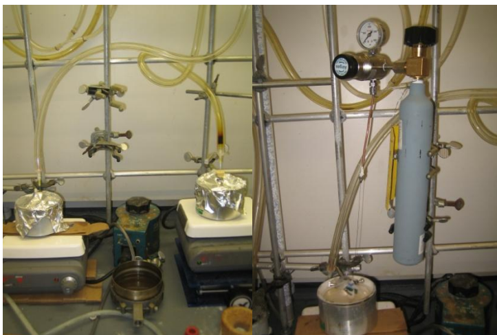
Figure 1. ^{18}\text{O}_2 Gas Addition Experimental Setup: Freeze-Pump-Thaw Cycles for Substrates and NIS Solution (left), and Back-Fill with ^{18}\text{O}_2 Following Final Thaw Cycle
