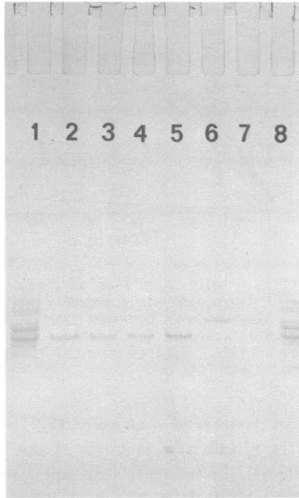
Fig. 3 A 20% polyacrylamide-urea gel after electrophoresis of tRNA samples. Slots 1 and 8 contain 3 \mu\text{g} of bulk tRNA from wild type S288C and 759-5B mia , respectively. About 0.3 \mu\text{g} of purified tRNA samples were applied to the remaining slots: 2) wild type tRNA Phe , 3) mia tRNA Phe isoacceptor A, 4) mia tRNA Phe isoacceptor B, 5) mia tRNA Phe isoacceptor C, 6) wild type tRNA Tyr , and 7) mia tRNA Tyr isoacceptor D.
