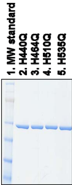
Supplementary Figure S4. SDS-PAGE analysis of HSA variants. Equal amounts (1 \mu\text{g} ) of HAS variants (H440Q, H464Q, H510Q and H535Q) were applied on a NuPAGE 4-12% Bis-Tris gel. Electrophoresis was performed for 50 min at 200 V. Gels were stained with InstantBlue protein stain (Expedeon).
