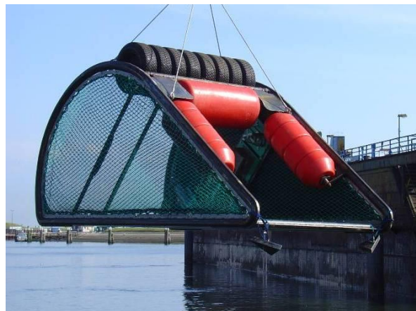
▲ Figure S1-3. SUIT frame with floats and side nets during a test deployment in the harbour of Texel (NL).
