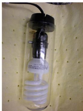
Pyrex glass tube encasement with rubber stopper
