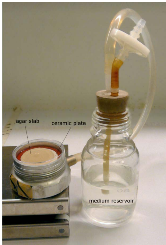
Supplementary Figure 1. Photograph of the agar-slab PSM system. Matric potential is manipulated by changing the relative elevation of the slab in its container with respect to the air / liquid interface in the medium reservoir.
