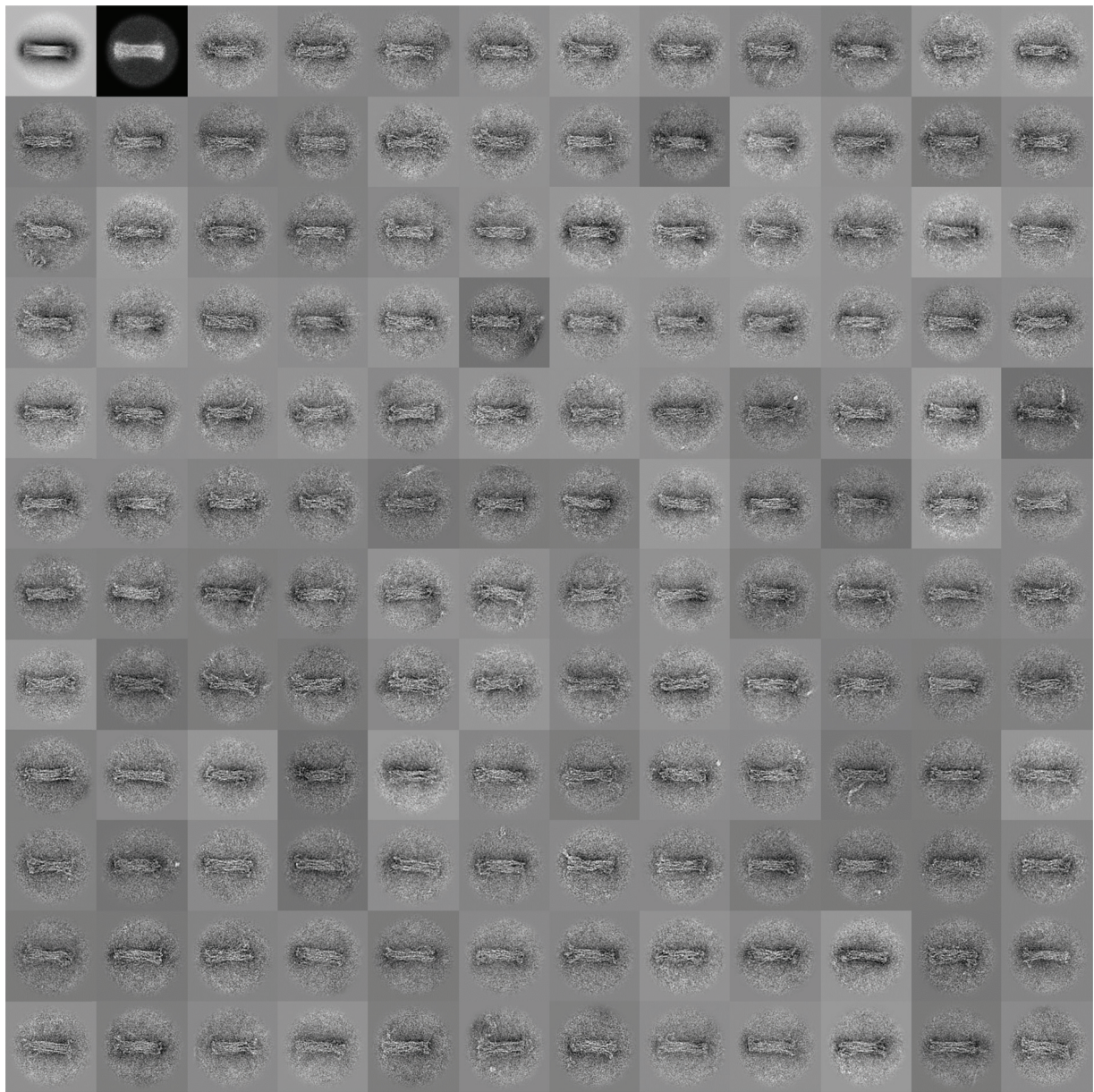
Figure S13 TEM images of the 32-helix bundle with a crossover spacing of 63 basepairs. The first two images show the mean and variance of 142 single-particle images.
