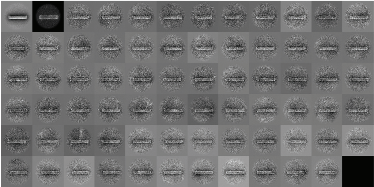
Figure S10 TEM images of the 32-helix bundle with a crossover spacing of 21 basepairs that exhibits a clear stripe pattern. The first two images correspond to the mean and variance of 69 single-particle images.
