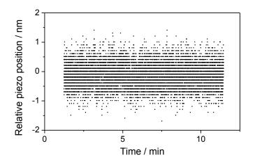
**Figure S-2.** Plot of relative piezo position read from the capacitive sensor of the positioner. The zero position corresponds to the position where the tip approach was stopped.
