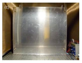
**Figure S-1.** Images of (a) SECM stage, tip, and cell, and the isothermal chamber closed (b) with (b) a VIP and then (c) with an aluminum plate.
