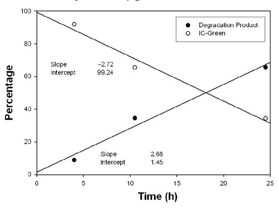
Supplemental Figure 1: An HPLC stability study of ICG in saline over a 25 hour period shows that ICG is unstable and rapidly forms degradation product.
