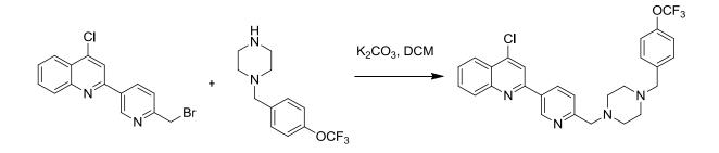
Quinoline **50** (0.40 mmol, 1 eq.) was added to DCM (20 mL) with 4-OCF<sub>3</sub>-benzylpiperazine (0.80 mmol, 2 eq.) and  $K_2CO_3$  (0.6 mmol, 1.5 eq.). The solution was allowed to stir at room temperature overnight. The salt precipitate was filtered off and the crude solid was purified by flash column chromatography (eluting with 100% EtOAc) to give the desired compound as a white solid.
