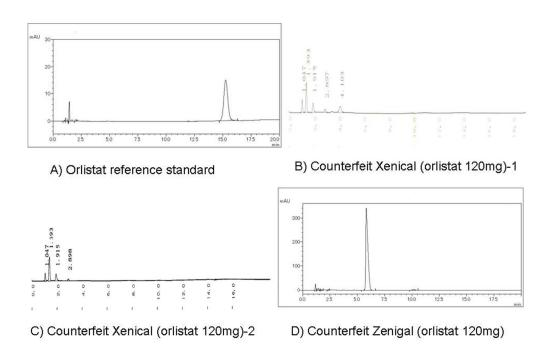
Figure 1: Chromatograms of the reference standard of orlistat and counterfeit samples 254x190mm~(96~x~96~DPI)
