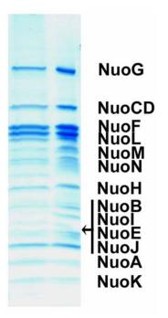
**Supplemental Figure 1. Purification of complex I from** *E. coli.* Coomassie Blue-stained SDS-PAGE gel from a sample of purified *E. coli.* complex I
