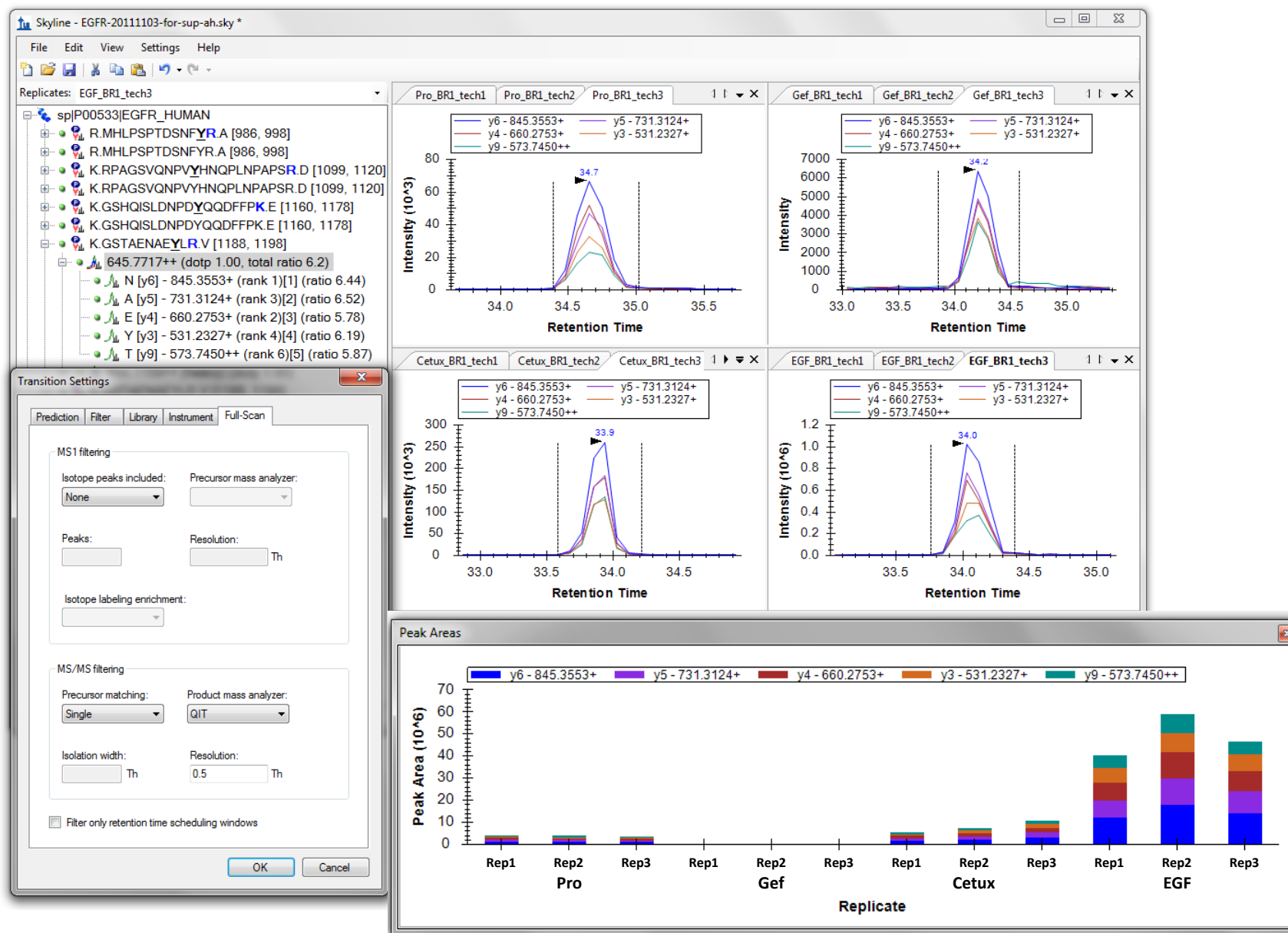
Supplemental figure S1. Skyline MS/MS settings, replicate peak areas and imported data from a targeted MS/MS from EGFR samples run on a Thermo Fisher LTQ-Velos, low resolution instrument. The differentially colored chromatographic traces are for the individual pSRM extracted transitions from the targeted MS/MS scans.
