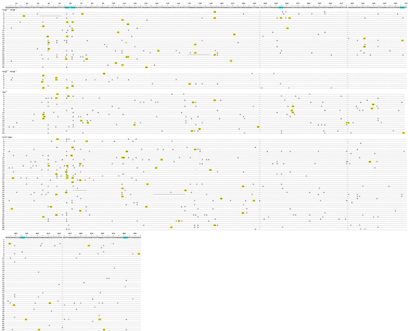
Figure S1. Location of tandems in the J_H4 intron. All J_H4 sequences that contain tandem mutations, highlighted in yellow, are aligned. WGCW hotspots are highlighted in the germline sequence in blue. Pol\zeta^{+/+} Pol\eta^{-/-} and Pol\zeta^{+/-} Pol\eta^{-/-} sequences are shown to base 370, as no tandems were found in bases 371–492. Ung^{-/-} sequence data were only available to base 368. Wild-type sequences are displayed through base 492 to show all tandems. In wild-type sequence 12, bases 315 and 316 are not considered a tandem as base 316 is an insertion. For the two triple tandems, the first and second bases were used for the spectra analysis. Dashes represent deletions or gaps corresponding to insertions in another sequence.
