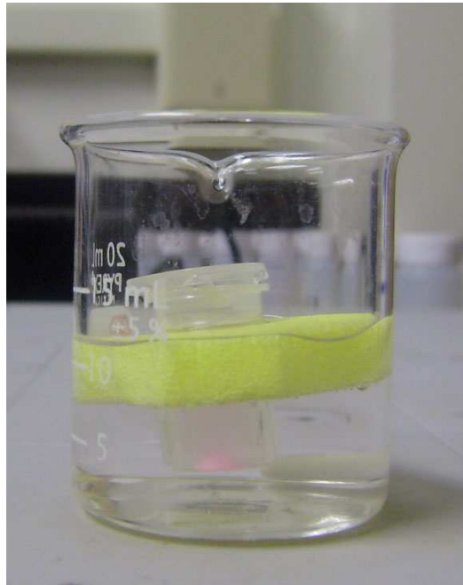
Figure S2. Set-up for Rh6G release test.
