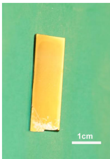
Figure S5. Photograph of (\text{AuNPs}/\text{CH})_{15} films deposited on a silicon wafer.
