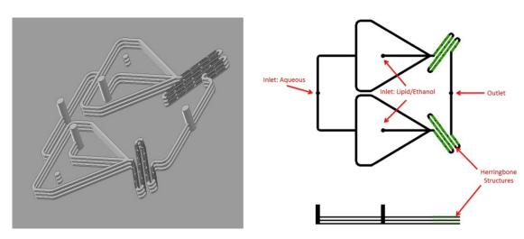
Supplementary Figure S3: Schematic of 6x scale-up microfluidic device for formulation of lipid nanoparticles using individual microfluidic SHM mixers. a.
