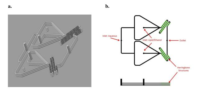
Supplementary Figure S3: Schematic of 6x scale-up microfluidic device for formulation of lipid nanoparticles using individual microfluidic SHM mixers. a. CAD drawing of 6x scale-up SHM. b. Schematic of 6x scale-up SHM.
