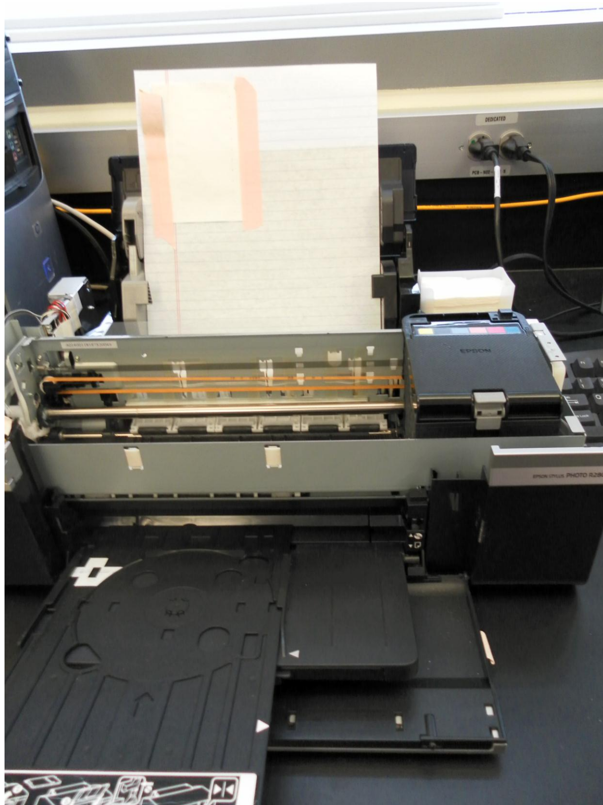
Figure S2. EPSON R280 inkjet modifications for printing carbohydrate bio-inks; uncovered printing mechanism including cartridges, inkjet, and DVS-activated sheet taped onto normal printer paper, ready to be printed with bio-ink.
