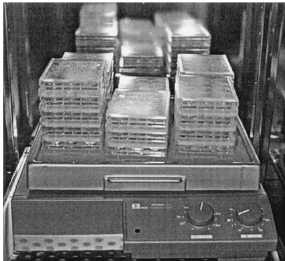
Figure 1. Shaken multi-well system. 12-well microtiter plates on a rotational shaker can readily simulate stirred tank bioreactor conditions. pH, temperature and humidity are controlled by a CO 2 -incubator. All transfection experiments were carried out in this system.
