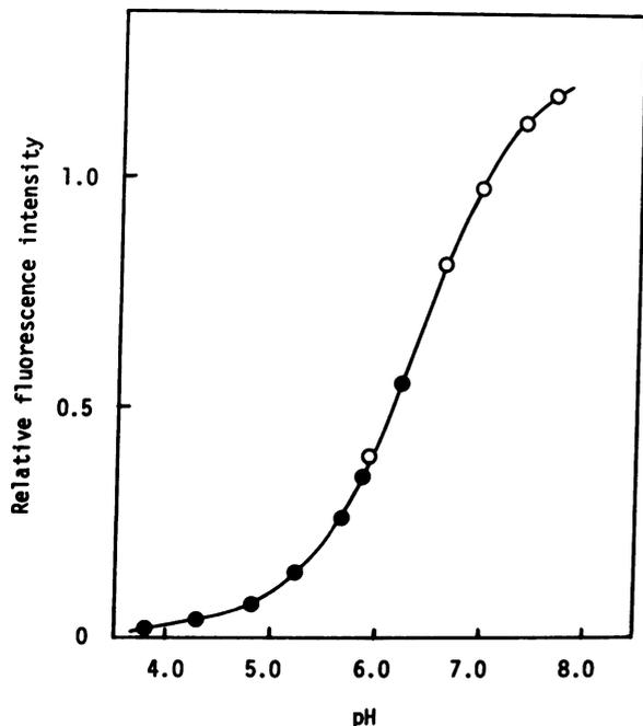
FIG. 1. Relative fluorescence intensity of FITC-dex at various pH values. Intensity at pH 7.0 is taken as unity. Excitation was at 495 nm and emission was measured at 550 nm with 5-nm slits on both monochromators. FITC-dex (1  $\mu$ g/ml) was in 50 mM NaCl/10 mM buffer (●, NaOAc; ○, Na phosphate).
