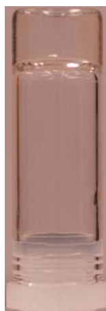
Figure S3. Optical image of the hydrogel of 1 in water (0.6 wt%, pH = 7.4).
