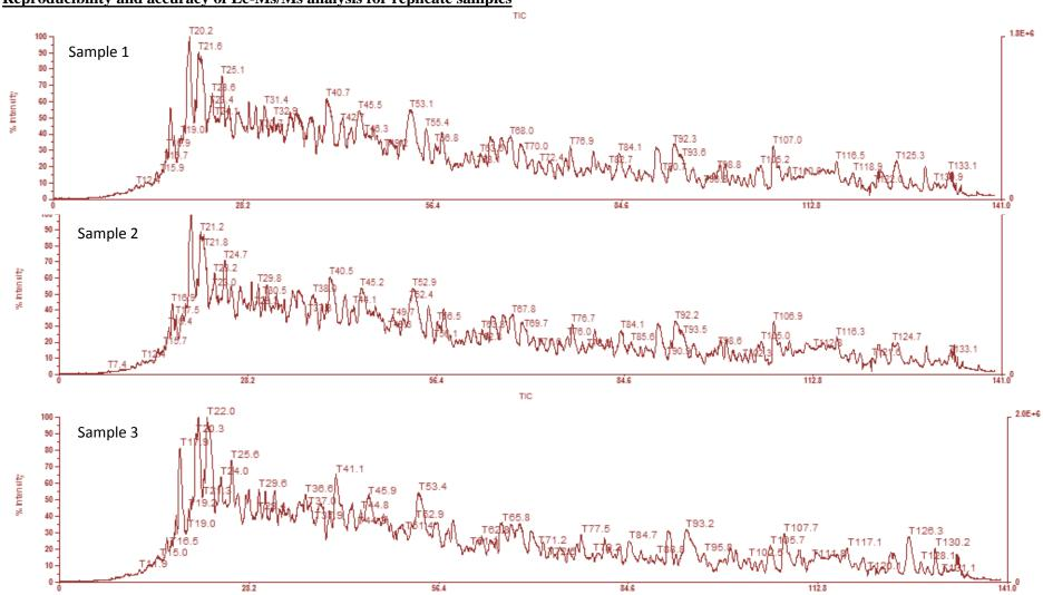
Illustration showing total ion chromatography (TIC) of colon samples used in current experiment. TIC showed a stable and consistent similarity reflecting stability of mass spectrometry. Attention was always monitored to achieve maximum reproducibility and minimizing any variation that might arise from experimental error. Figures were captured using Hitachi NanoFrontier LD data processing software, Tokyo, Japan.
