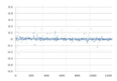
Accuracy of mass spectrometry was confirmed when blotting the delta mass ( $\Delta$  max); differences between theoretical (Th Mw) and calculated molecular weight (Calc Mw). Shift in most cases were within 0.05 as shown above.
