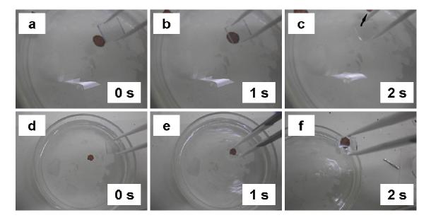
Additional file 1. Comparation of ITO substrates before and after modification by chloroform. Before modification, when ITO substrate approach P3HT pillar film reverse side (a, b), the film was pushed away (c). After modification, when ITO substrate approach P3HT pillar film reverse side (d, e), the film was attached to the substrate (f).
