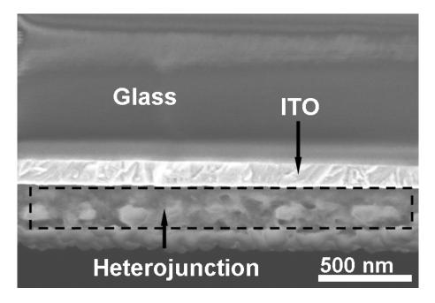
Additional file 3. (Cross section) SEM image of P3HT/  $C_{60}$  heterojunction. It also shows the thickness of heterojunction is less than 200 nm.
