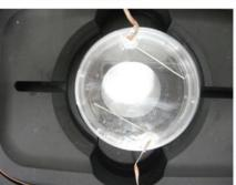
**SUPPLEMENTARY FIG. S2.** (A) The apparatus used to electrically stimulate engineered C2C12 muscle tissue. (B) The design of the *in situ* chamber ( $37^{\circ}$ C, 5% CO<sub>2</sub> atmosphere) ensured the long-term viability of the myotubes. Long Pt wires that served as electrodes were placed inside the Petri dish near the muscle tissue. This arrangement effectively increased the efficiency of the applied electric field.
