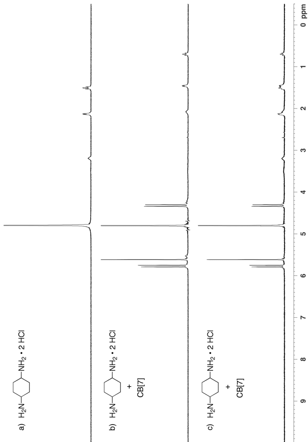
Figure S45. ^1\text{H} NMR spectra recorded ( \text{D}_2\text{O} , 400 MHz, RT) for : a) 7 (0.5 mM), b) a 1:1 mixture of CB[7] (0.5 mM) and 7 (0.5 mM), and c) a 1:2 mixture of CB[7] (0.5 mM) and 7 (1 mM).
