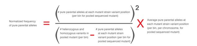
**Figure S4** *Variant Discovery Mapping* normalization equation. Pure parental alleles are defined as those positions in the pooled sequenced mutant where variant reads/total reads = 1 (after the appropriate variant subtraction strategy has been applied). Normalization is applied by default although users have the option of turning it off.
