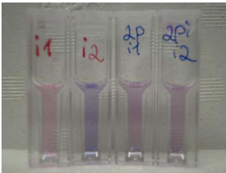
Figure 11. Comparison of the absorbance properties of TMR-MG dyes in PBS + , pH=7.4: TMR-2p-MG dyes have very similar absorbance while TMR- meta -MG and TMR- para -MG are very different
