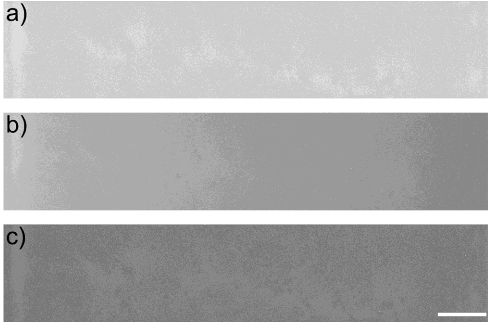
Figure S-2. Fluorescence micrographs of a segment of the gradient channel with a solution of RTDP in a PBS buffer in water taken at different [O_2] in the gas channels of the microfluidic device. The field of view is 500 \times 100 \mu\text{m} . The images are flat-field corrected to compensate for unevenness of the illumination and light collection. (a) [O_2]_A = [O_2]_B = [O_2]_C = 0 (pure N_2 in all gas channels), resulting in [O_2] = 0 everywhere in the gradient channel. (b) [O_2]_A = 0 , [O_2]_B = 20.8\% , and [O_2]_C = 10.4\% , resulting in [O_2] linearly varying from \sim 3.3\% to \sim 17.5\% across the gradient channel. (c) [O_2]_A = [O_2]_B = [O_2]_C = 20.8 (air in all gas channels), resulting in [O_2] = 20.8\% everywhere in the gradient channel. We note that, because RTDP was dissolved in water (rather than 66% solution of ethanol in water), the \sim 14\% variation of [O_2] across the gradient channel in b , corresponded to a change of only \sim 31\% in the RTDP fluorescence. Scale bar 50 \mu\text{m} .
