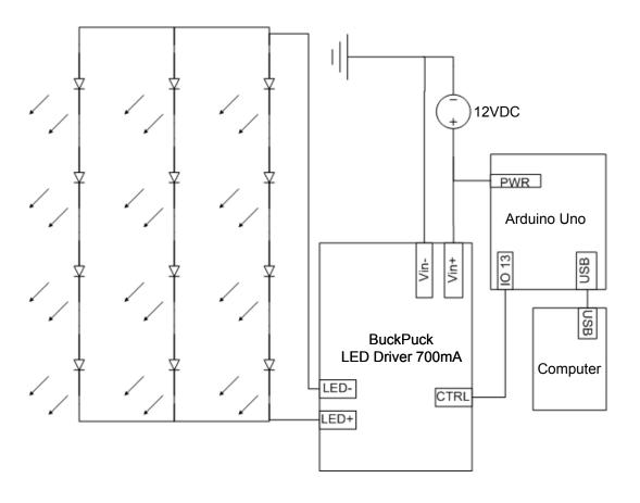
Supplemental Figure 2. Diagram of blue LED control circuit.
