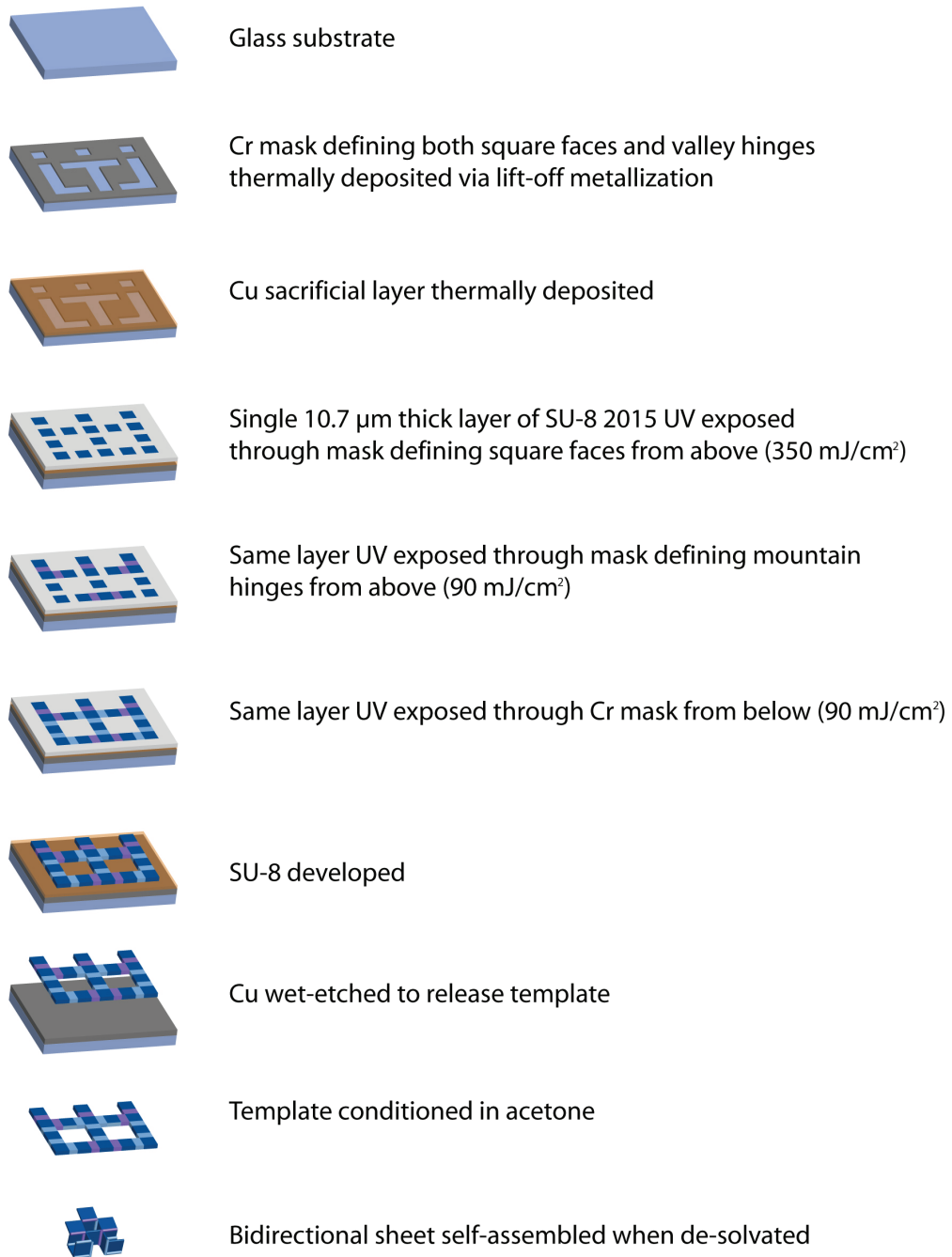
Supplementary Figure S9. Schematic illustration of the fabrication steps for self-assembling bidirectional sheets (Figs. 3c,e,f, main text).
